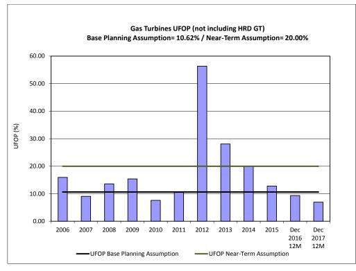
Figure 3 Gas Turbine UFOP – HWD/HVY/SVL Units
